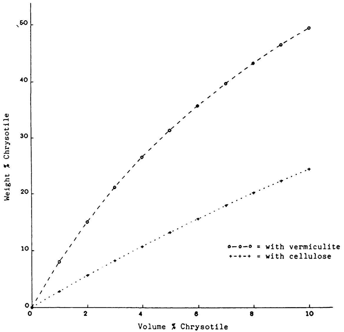
Figure C1. Relationship between volume % and weight % of chrysotile mixed with a)vermiculite and b) cellulose.
